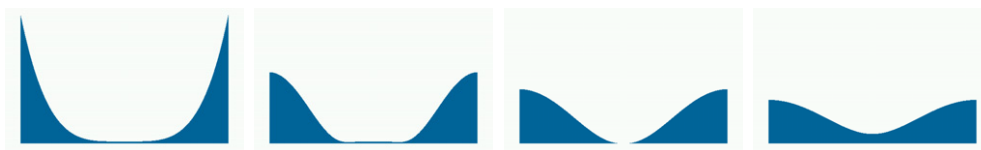
Figure 2. Dead core phenomenon: the snapshots show a solution to the equation u_t + \partial_x(uu_{xxx}) = 0 on the interval [0, 1] . The first picture shows the initial data, u_0(x) = (x - 0.5)^4 + 0.001 ; the subsequent ones the solution at times t = 0.002, 0.012 and 0.040 . Although initial data are strictly positive, the solution does not stay strictly positive at all times.
